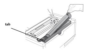
5. Lower the right side, aligning the lock lever slot with the ridge in the drum cartridge.
