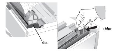
6. When the cartridge is in place, push the lock lever forward until it stops.
