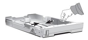
3. Fan a stack of paper (Maximum 250 sheets, 20 lb.) and place it in the tray under the tabs. Do not fill above the "PAPER FULL" mark. To use letterhead, place paper print side down, top-edge facing you.
