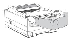
2. Lift out the image drum cartridge. **Do not touch the drum's green surface**.
