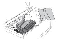
4. Remove the new image drum cartridge from the package. To install the new image drum cartridge, follow the installation instructions in Section 1 (or the instructions included in the replacement kit).
