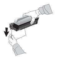
4. Reinstall the image drum cartridge in the printer.
