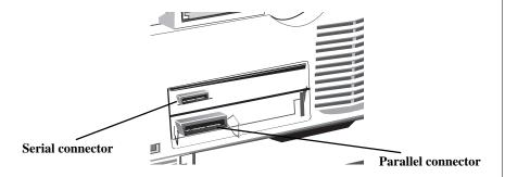
2. Connect the other end of the cable to the proper connector on your computer. Fasten the cable securely to your computer.
